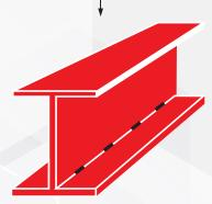
H-beam assembling (by auto Spot Welding)
